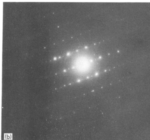
Figure 7 Cleaved fibrillar section of a macroscopic pTS crystal. (a) Typical area. (b) SADP from doubly exposed area in (a) showing that chain direction is parallel to the fibril axis.
